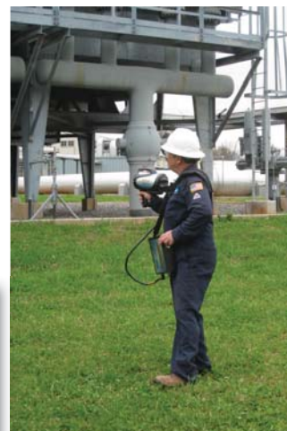
Technician utilizes Heath's RMLD® to screen a piping facility.
