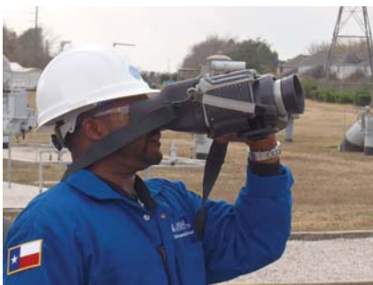
Technician Performing Survey utilizing EYE-C-GAS™ Imaging Camera
