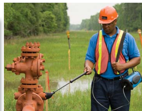
Heath's DP-IR™ intrinsic safety rating makes this the perfect instrument for the inspection of an above ground block valve.
